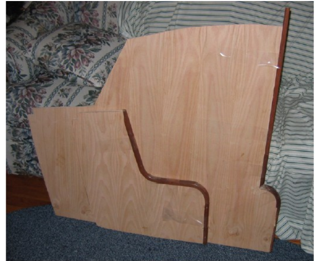
In this photo, one can see my clamping method for gluing the trim boards. It was actually strong, clear and stretchable tape.
