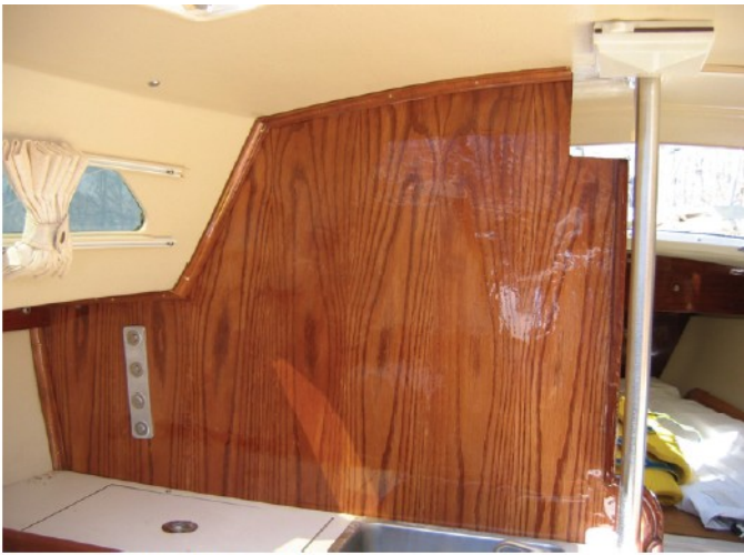
New port bulkhead looking from the stern.
