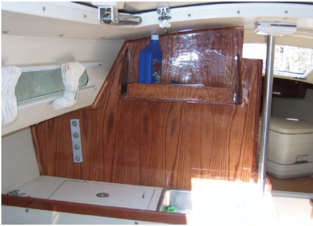
Port Bulkhead from stern with shelf. This photo also shows the aluminum backing plate for the chain plate bolts.
