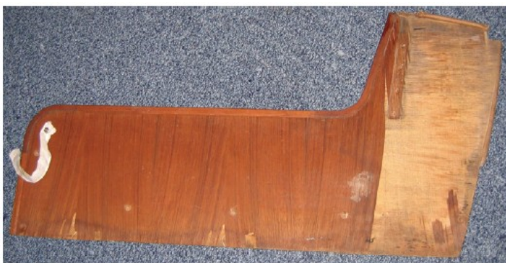
Old port bulkhead showing the rot on the bottom and the missing veneer (Not all of this veneer was missing when I bought the boat. Some started to fall off later).
