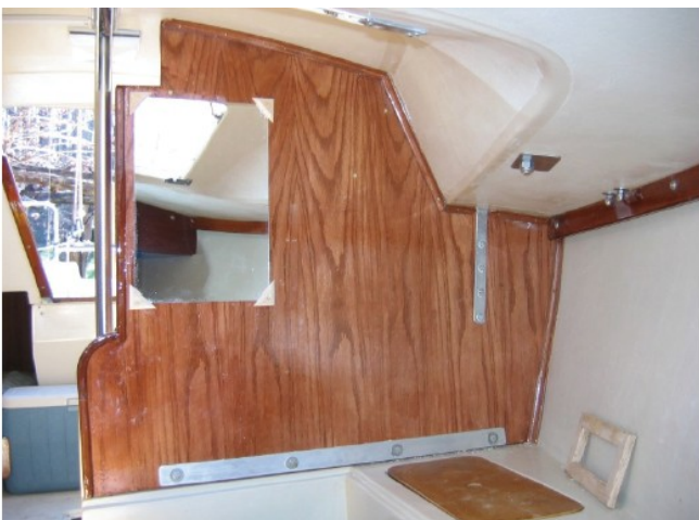
Port bulkhead from bow showing the Plexiglas mirror. This photo also shows the aluminum strap on the bottom edge of this bulkhead.
