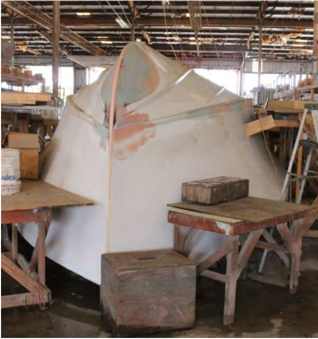
Below: an incomplete hull for the Catalina 545. The 545 was the new flagship for Catalina Yachts.
