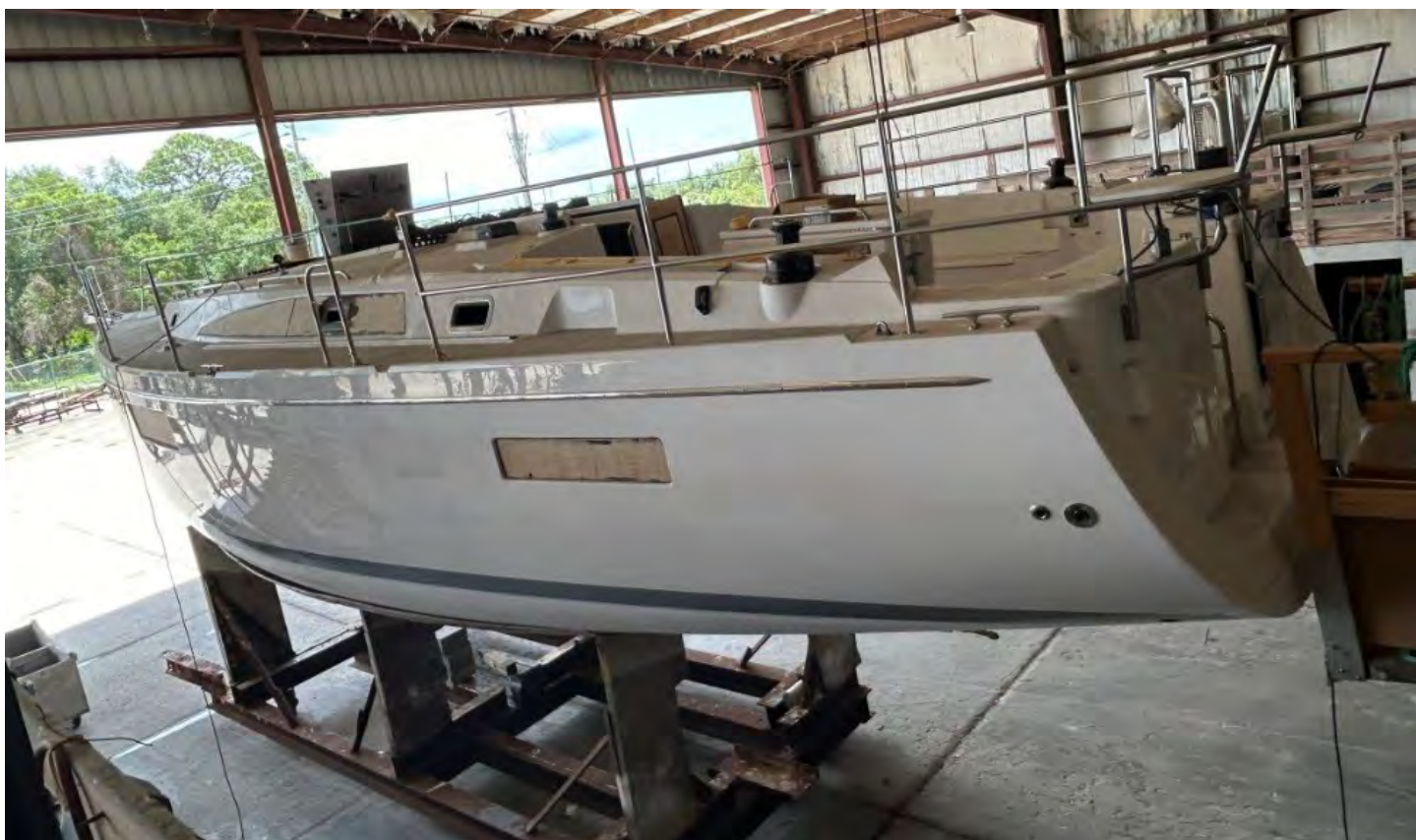
Above: Catalina 426, hull number 122, mostly complete. No keel or mast.
