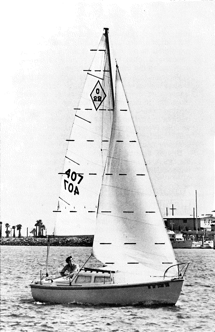
FIGURE 1 To illustrate the theoretical distribution of telltales on the sails, the editor has used a marking pen and ruled them in on an old photo of his boat.
