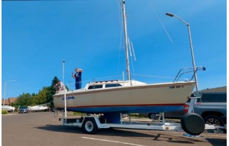
That is it, your mast is up you so now you just have to tune (tighten) the turnbuckles and you are off to the rest of the rigging for the day (boom, sails, BBQ, fenders, etc....). Pro Tip: Clothes pins work great to hold up your shroud covers.
