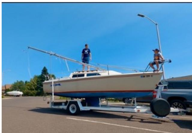
3. Check your rigging. Check all your stays, lines, halyards, straps, etc. to make sure they will not snag. On a Catalina 22 the turnbuckles are common snag points for the side stays (shrouds). Pro Tip: use a small piece of line tied through the lower toggle to prohibit it from falling to the side and preventing the turnbuckle from rotating properly (thanks Don Boyko for that one).
