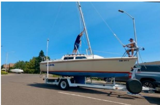
5. Lift smoothly and fully. Complete the lift if you can in one smooth movement. This may mean you need to stand on the cabin top to make the lift easier. It may mean you have to have help lifting. No matter what your plan is make sure the mast is lifted smoothly and fully before you start to relax. I have been there and watched a mast come back down when someone let go about 3/4 of the way up when they thought someone else had it and let me tell you it is a scary thing.
