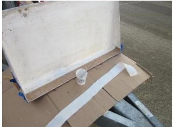
To eliminate the problem I removed the hatch and using my Dremel Tool with a grinding bit, I ground all the paint off along the front lip back several inches.
